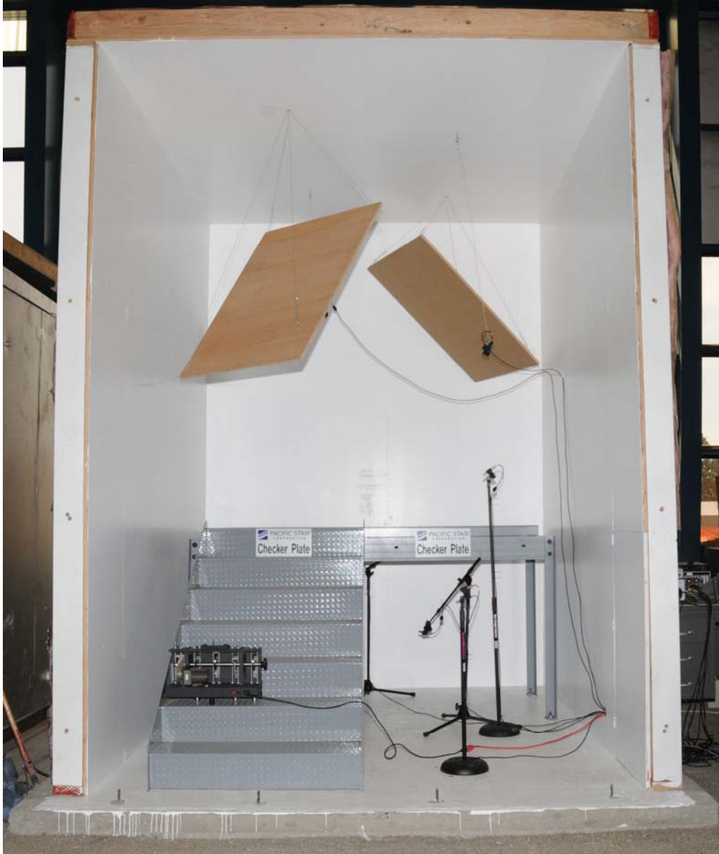
Fig. 1- Reverberation chamber with stair and landing assembly, standardized tapping machine, and microphone positions (front door is open).
