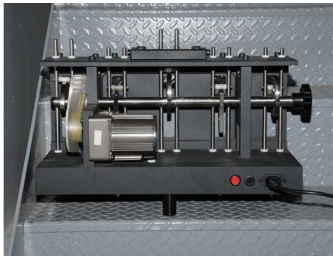
Fig. 4 – ISO Standard tapping machine placed on stair step.
